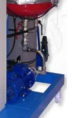
The Primer Station DPR is used for mixing a polyurethane distributed on the lower sheet of a sandwich panel as a thin layer (film).
