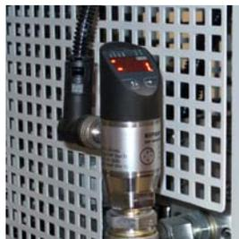
4. Overpressure Safety Gauge with divider
